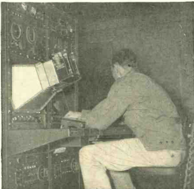
Receiver console and antenna of the SCR-270-D radar used by the Bureau of Standards to track meteors. The hooded equipment is the camera.
